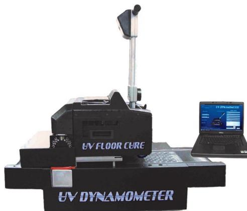
The Dyno has three axes: conveyor (controls the feed or cure rate), height (controls focus of lamp), and left/right slide rail (analyzes edge cure). USB ports on both pieces of equipment are used to connect to the laptop computer, which is part of the system, in order to control the process through the special software developed by HIDUV.
